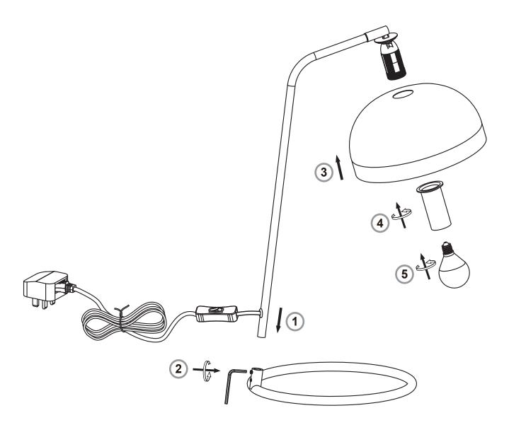
Grub screw can be adjusted and retightened to ensure the cable is at back of product when assembled.
